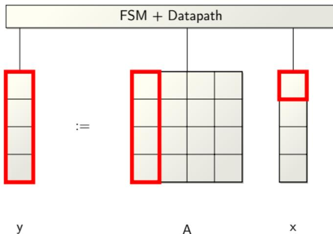
Arrays are implemented as block RAM, two data ports max.
